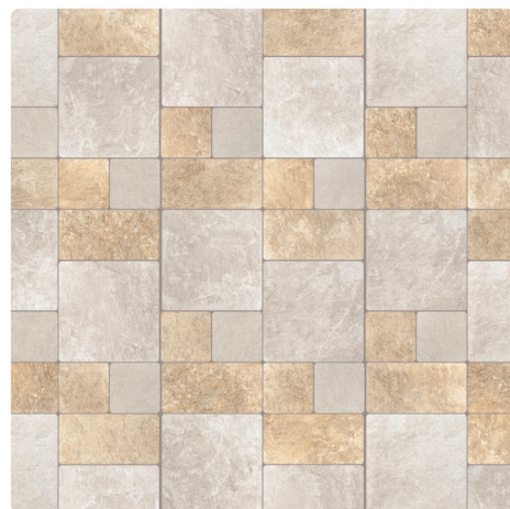
3COL-MIX-A.0101 23"x23" 11 1/2"x23" 11 1/2"x11 1/2" MOD.27 / SOFT MATCHING / EARTH MODULE % INDIANA BUFF SELECT 12,5% TRAVERTINE CROSS CUT WHITE 50% TRAVERTINE CROSS CUT CREAM 25% 12,5%
